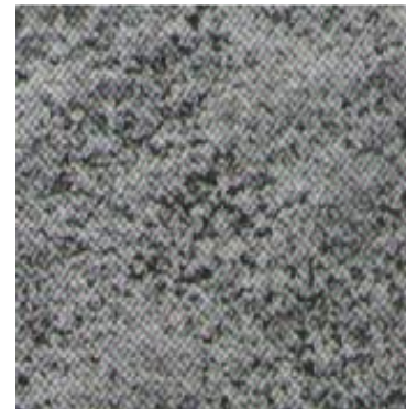
SEM of a sintered bead porous surface
