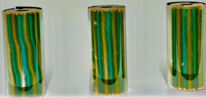
32-pole outer rotor for stepping motor
